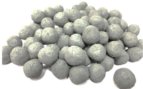
For several years of experiments at the facilities of some mining companies, a universal binder has been created that can be used on any iron ore concentrate. The binder of our company can be used as the only binder, instead of bentonite clay.
